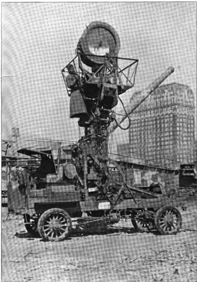
The projector is mounted on a turntable and is electrically operated so that it may be swung on both a horizontal and vertical axis, the movement being controlled from a distance of 500 feet. The arm is raised by a mechanism operated from a power take-off from the driving shaft of the chassis. It is provided with safety devices, controls, etc. It operates rapidly and throws a powerful light for a distance of many miles.
